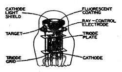
FIG. 34—Internal construction of electron ray indicator tube. (Courtesy R.C.A. Mfg. Co. Inc.)
