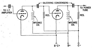
FIG. 31—Inter-stage coupling in an impedance coupled audio frequency amplifier.
