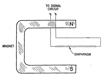
FIG. 10—Principal element of metal strip speaker. A megaphone is usually associated with this type of speaker.
