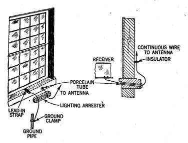
FIG. 8-Conventional method of installing inverted L-antenna lead-ins.
