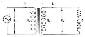
FIG. 4—Simple diagrammatical representation of typical transformer.
