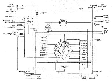
FIG. 5-Internal connection diagram of Weston Model 665 selective analyzer.
