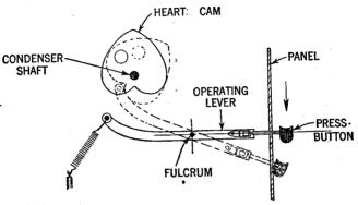
FIG. 8—Principles of control in which the tuning condenser is rotated by the pressure of a lever against a heart cam.
