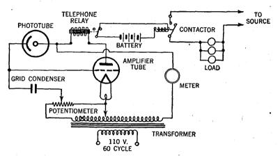
Fig. 2.—Circuit showing typical connection when it is necessary to operate a larger load than is possible when using only a communication type relay.
