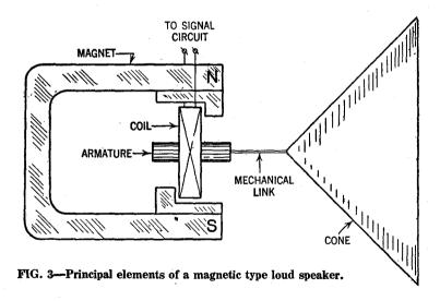
Magnetic Speakers.—In this type the moving iron driving type is employed. The principle of operation is based on the varying of the magnetic polarity of the armature. These variations are caused by the electrical impulses flowing through the coil winding which encircles the armature.
