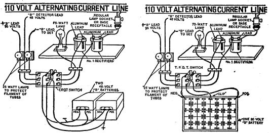
Fig. 23.—Diagram showing charging switch circuit for two 48 volt units.
