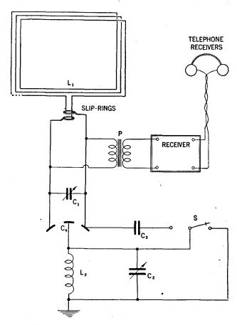
FIG. 4-Circuit of Kolster radio direction finder.
