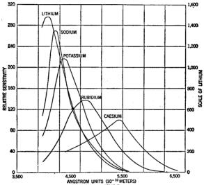
Fig. 3.—Curves showing color sensitivity of various elements.
