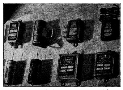
FIGS. 13 to 22-Various types of condensers used in radio work.
