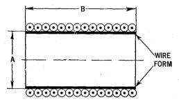
FIG. 1-Cross-section of single layer coil.
