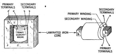
FIGS. 7 and 8—Shell and open core type transformers having the primary and the secondary winding placed directly on top of each other.
