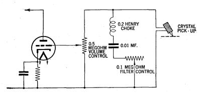
FIG. 13-Method of connection for phonograph pick-up.
