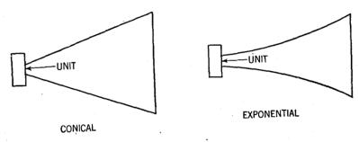
FIGS. 1 and 2-Conical and exponential horn forms.
