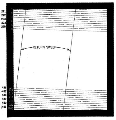
FIG. 20—Illustrating principles involved in establishment of an interlaced scanned picture.
