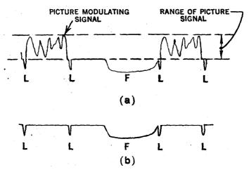
FIG. 19—a, composite signal containing picture modulation and synchronizing impulses; L, line synchronizing; F, picture frame synchronizing; b, synchronizing impulses applied to saw-tooth generators.
