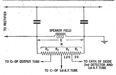
FIG. 41—Method of obtaining grid bias by utilizing voltage drop across speaker field coil.
