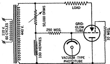
Fig. 47.—Grid-Glow relay circuit A. C. operation.
