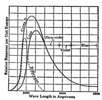
Fig. 12.—Spectral characteristics for a caesium-oxide phototube.
