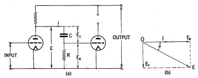
Fig. 17.—Showing interstage coupling and efficiency components with vector diagram.
