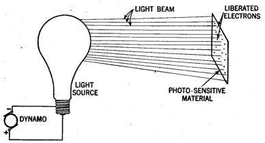
Fig. 1.—Illustrating how a body consisting of photo-sensitive material emits electrons by means of light.
