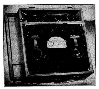
FIG. 26-Exterior view of Supreme Model 551 analyzer.
