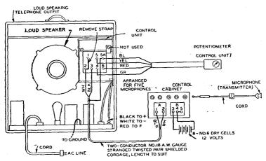
FIG. 2-A small portable announcing system.
