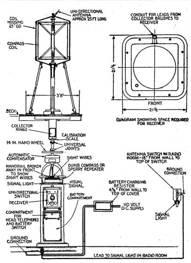
FIG. 3-Kolster radio compass installation.
