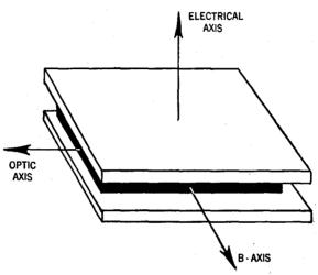
FIG. 13-Mounting of the crystal.
