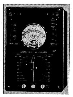
FIG. 4-Front view of Weston Model 665 selective analyzer.
