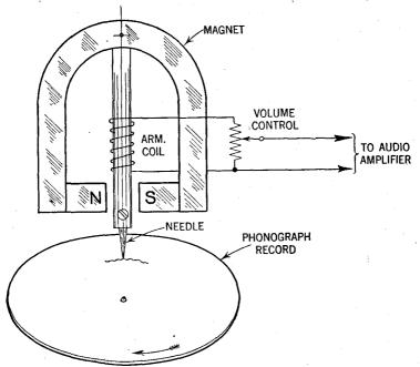
FIG. 3—Simplified layout of a phonograph pick-up.
