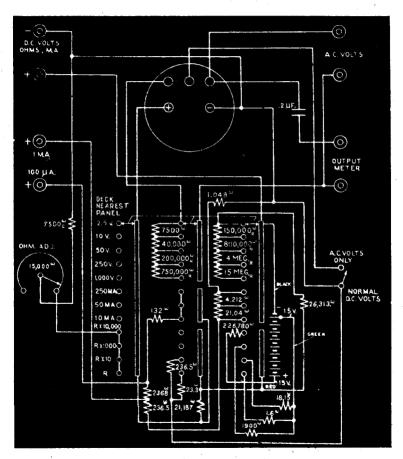
FIG. 14-Wiring diagram of Weston Model 772 analyzer.
