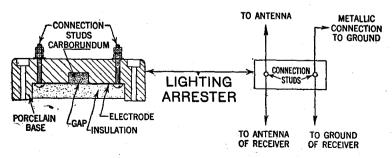
FIG. 9-Lightning arrester detail and diagram of connection.
