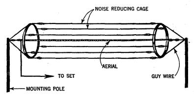
FIG. 15-Cage antenna. A type frequently used at transmitting stations.
