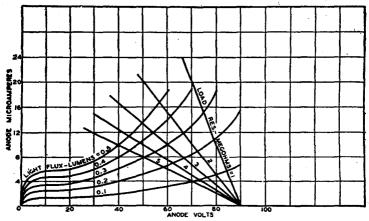
Fig. 7.—Average gaseous type anode characteristics.
