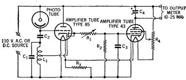
Fig. 24.—Circuit for measurement of small amount of light.
