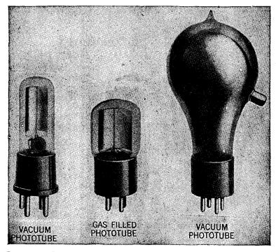
Fig. 5.—Typical phototubes.
