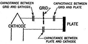
Fig. 16.—Diagram showing inter-electrode capacitances in a triode.
