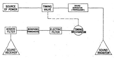
FIG. 18—Diagram showing co-ordination of apparatus usually employed in Sonic airplane altimeters.
