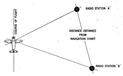
FIG. 6—Illustrating method of determining position by means of radio compass. As the surrounding territory shown on air navigation chart is laid out in scale, it follows that the intersection of the two lines gives the approximate location of the aircraft. It is evident that the accuracy of position so obtained will depend on such factors as: flying speed; angle and distance between aircraft and stations; accuracy of instruments; skill of navigator, etc.
