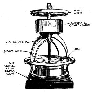
FIG. 8-Kolster compass and compensator arrangement.
