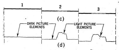
FIG. 16—Showing fundamental scanning principles.
