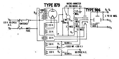
FIG. 10-Typical circuit for cathode ray oscillograph.
