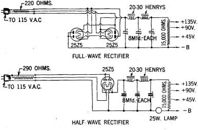
FIGS. 12 and 13—Illustrates two transformerless power supplies, for full-wave and half-wave rectification respectively. Here a line cord resistor is utilized to drop the line voltage to that necessary for the filaments of 25Z5 tubes. The third element in the line cord resistor brings the full line voltage for the plate of the tubes.
