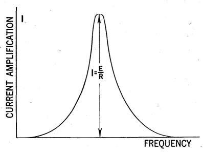
FIG. 5-Typical current resonance characteristic.
