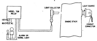
Fig. 4.—Diagram illustrating typical connection of equipment shown in figs. 1 to 3.
