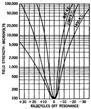
FIG. 5-A typical radio receiver selectivity curve.
