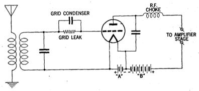
FIG. 26-Detector circuit grid-leak and condenser method.
