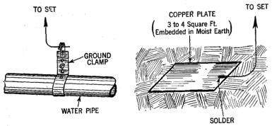
FIGS. 10 and 11-Two methods of ground connection.
