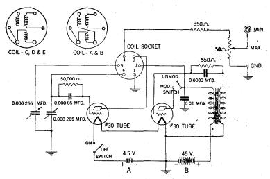
FIG. 39—Wiring diagram and coil arrangement in Readrite Model 557 signal generator.
