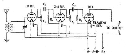
FIG. 13-Two stage impedance coupled radio frequency amplifier.
