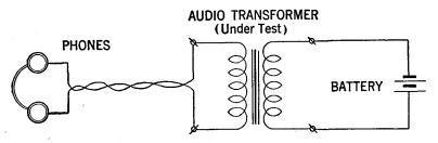
FIG. 18-Method of detecting trouble in audio transformer.
