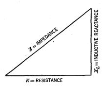
FIG. 11.—Illustrates vector relation between the inductive reactance and the resistance. To obtain the impedance: Resistance R (in ohms) is laid off horizontally; the inductive reactance RL(also in ohms) is laid off to form the perpendicular. Measure the hypotenuse (in the same scale) which gives the impedance of the circuit in ohms. This triangle is variously referred to as the impedance triangle, vector diagram or impedance calculator.
