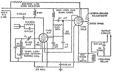
Fig. 38.—Self-balancing capacity-operated relay.
