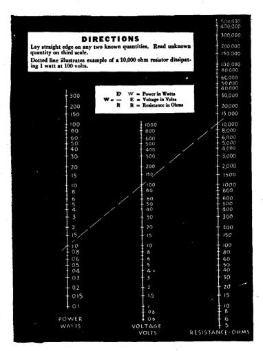
FIG. 24—Convenient table giving the scalear relation between resistance (R), voltage (E) and power (W). With the chart and a straight edge any of the above quantities can be determined if the other two are known.
