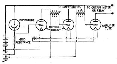
Fig. 7.—Transformer coupled multi-stage amplifier for use with photo-electric tube.
