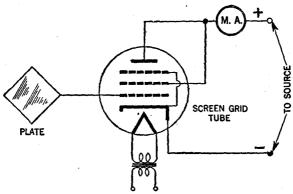
Fig. 36.—Simple circuit for capacity indications.
