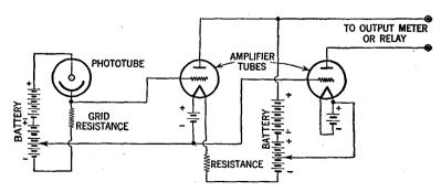
Fig. 9.—Resistance-coupled multistage amplifier for use with photo-electric tube.
