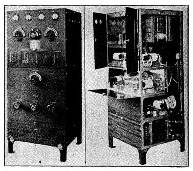
FIG. 2-Standard 200 Watts Marine Radiobeacon transmitter.
