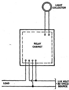
Fig. 6.-Wiring diagram of illumination control unit.
