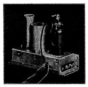
FIG. 15—Exterior view of typical oscillator unit.
