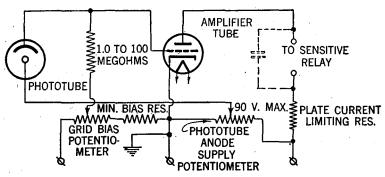
Fig. 27.—Typical relay circuit employing gaseous type phototube.
