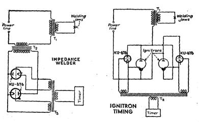
Figs. 6 and 7.—Illustrates the connection of 2 thyratron tubes in welding applications.
