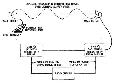
Fig. 35.—Elementary diagram of connection between the principal units used in radio receiver remote control.
