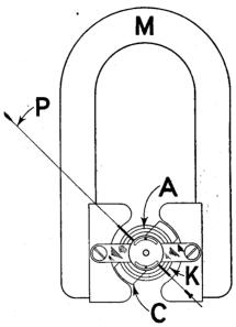
FIG. 6—The essential parts of the instrument are: A, spiral spring; C, coil; K, soft iron core; M, permanent magnet and P, pointer. Current passing through the coil causes the moving system to turn against the restraining force due to the influence of the permanent magnet.
