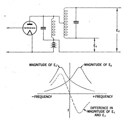
FIG. 2—Diagram and plotted curves illustrating how the potentials at either end of secondary are 180° out of phase.
