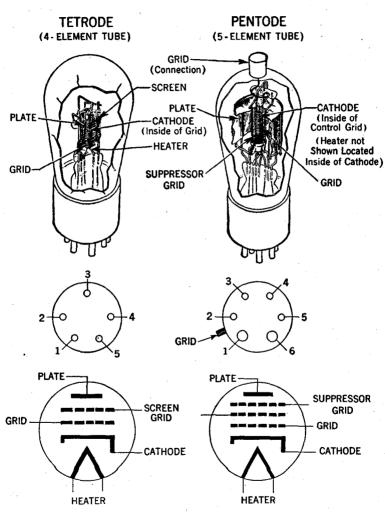
Fig. 7.—Views of four and five element vacuum tubes, showing arrangement of prongs and wiring symbols.
