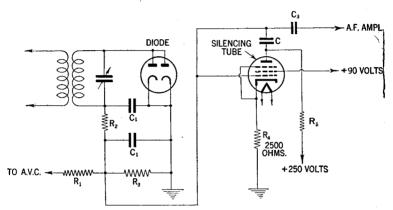
FIG. 14-Automatic tone control circuit.
