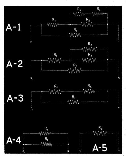
Method illustrating how a series parallel resistance combination of type shown in A-I may be reduced to the simple form of that shown in fig. A-5.
