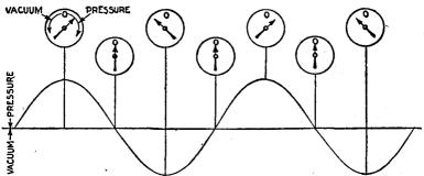
Fig. 3.—Diagram illustrating pressure variations due to sound waves. It should be noted that the type gauges shown, register pressure above atmospheric when the pointermoves to the right of the vertical, and vacuum or pressure below atmospheric when it moves to the left of the vertical.
