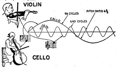
Fig. 9.—Properties of wave motion illustrating pitch.
