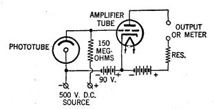
Fig. 28.—Typical high-voltage circuit providing over-voltage protection for phototube.
