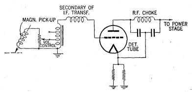
FIG. 10-Method of radio phonograph pick-up connection.
