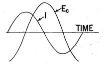
FIG. 3-Voltage and current vectors for a circuit containing resistance and capacity in series.
