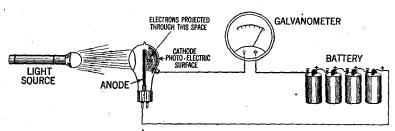
FIG. 2—To increase the amount of deflection (efficiency of light conversion) various methods of current amplification similar to that associated with current amplification in radio circuits is employed.
