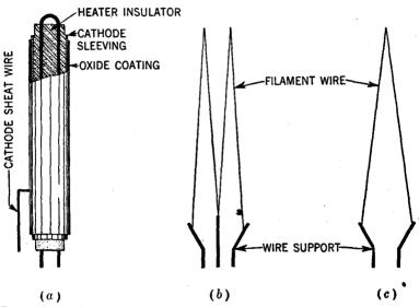
Fig. 8.—Schematic diagram of directly and indirectly heated cathodes.
