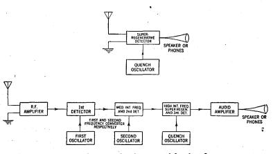
FIGS. 3 and 4—Block diagrams showing essential units of a super-regenerative and a super-infra regenerative circuit respectively.
