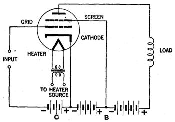
Fig. 17.—Connection of electrodes of a screen gride tube.
