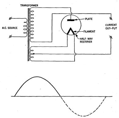
FIG. 11.—Connection diagram of the half-wave rectifier. The rectified current is depicted on the upper half of the wave diagram.
