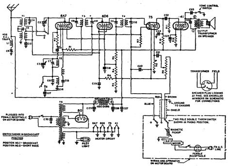
Frg. 20.—Circuit diagram of a 5-tube combination phonograph and dual-wave superheterodyne receiver. (Emerson Model L-143.) I.f. peaked at 456 kilocycles. Voltage rating 105 to 125 volts a.c. Current drain 0.5 amperes for receiver. Frequency range 540 to 1,750 kilocycles—2,200 to 7,500 kilocycles. Speed of phonograph motor 78 r.p.m. at 105 to 125 volts, 60 cycle a.c. supply.
