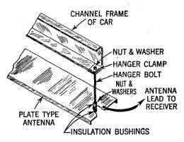
FIG. 3—Showing method of fastening plate-type antenna to channel frame of car.
