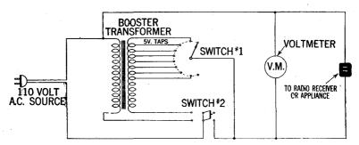
FIG. 17-Schematic diagram of voltage compensating equipment.
