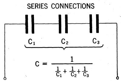
FIG. 9—Mathematical relation between the total capacitance and the individual capacities when connected in series combination.
