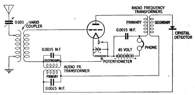
FIG. 28-Diagram showing typical reflex circuit.
