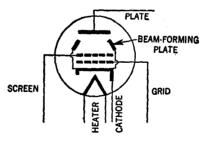
Fig. 19.—Conventional representation of beam power tube.
