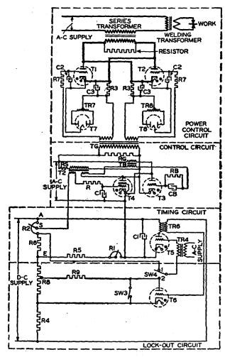
Fig. 10.—Schematic circuit diagram of electrone tube welder control panel shown on opposite page.
