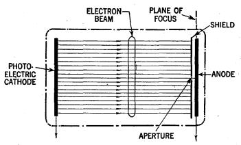
FIG. 23—Principle elements of Fansworth's "image-dissector" transmitting tube.
