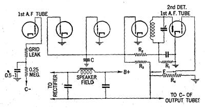
FIGS. 42 and 43—Grid bias method when receiver is equipped with automati volume control.
