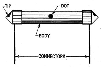
FIG. 23—Illustrating Standard Radio Manufacturer's Association (R.M.A.) color code for carbon resistance.
