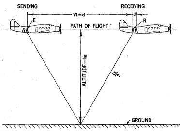
FIG. 17—Conventional geometrical representation for calculation of actual altitude of airplane.
