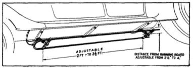
FIG. 5-Di-pole antenna and method of assembly.
