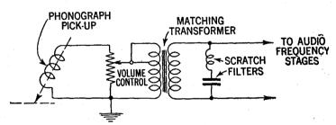
FIG. 11-Method of connection for a needle scratch filter.
