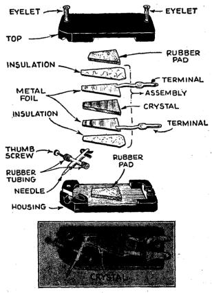
FIG. 6-Parts and assembly of crystal pick-up.
