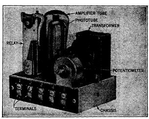
Figs. 3 and 4.—An A. C. operated photo-electric relay and connection diagram. A relay of this type may be used in automatic weighing processes; in machines for grading ball bearings; for the automatic inspection of vent holes in battery caps, and in many other applications.
