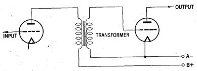
FIG. 32—Method of inter-stage connection of transformer coupled audio ferquency amplifier.
