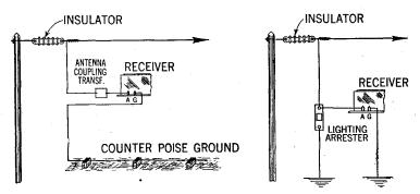
FIG. 12—Counterpoise and connection. Theoretically the counterpoise forms one plate of a condenser of which the main aerial is the other plate.
