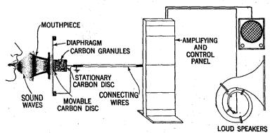
FIG. 6—Illustrating principal parts of a public address system.
