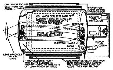
FIG. 30—Pictorial diagram explaining the action of the Fansworth television image dissector camera shown on page 592. It should be noted that the number of scanning lines is the horizontal frequency divided by the vertical frequency or Lines =  $\frac{\text{Horizontal frequency}}{\text{Vertical frequency}}$
