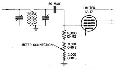
FIG. 9—Limiter circuit used in certain Pilot frequency modulation receivers.
