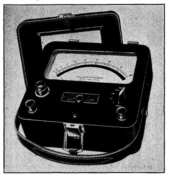
FIG. 17a-Weston Model 622 Thermo A.C.-D.C. Milliammeter.
