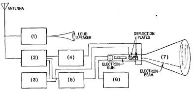
FIG. 7—Block diagram indicating fundamental unit that makes up a television receiver.
