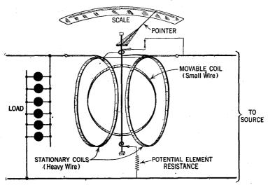
FIG. 20—Construction method of an electro-dynamometer as arranged to read watts.
