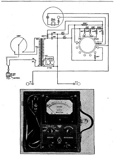
FIGS. 23 and 24—Schematic circuit arrangement and front view of typical ohmmeter.
