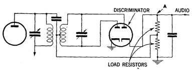
FIG. 11—Typical discriminator circuit. The demodulator of the frequency modulation receiver.
