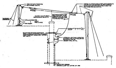
FIG. 18—Substantial antenna construction suitable for apartment house, school or hotel.
