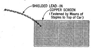
FIG. 1—A roof type antenna of this type consists of two copper screens fastened to cardboards and insulated from contact with car body.
