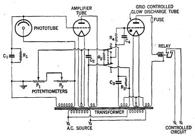
Fig. 10.—Wiring diagram of relay shown in fig. 9.
