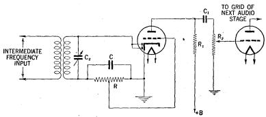
FIG. 23-Diode-biased detector circuit.
