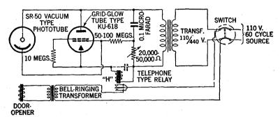
Fig. 34.—Diagram of connections for apparatus suitable to operate garage doors. (Circuit values are approximate only and may be adjusted if required).
