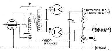
FIG. 3-Automatic radio frequency control detector diagram.
