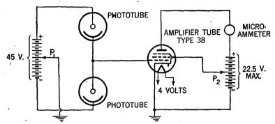
Fig. 22.—Sensitive circuit for matching measurement. Note:  $P_1$  should be set so that with no light on the phototubes, the output-meter reading is approximately mid-scale. Contact  $P_1$  should be set so that the maximum possible output current is limited to 100 micro-amperes.
