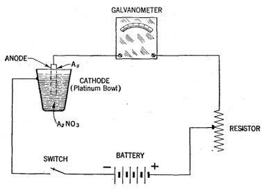
FIG. 5—Diagram of connection to obtain current strength by use of a silver-voltameter. *Example*: What is the current strength in amperes when after 20 minutes the silver deposit on the cathode is found to be 1.34 gram.
