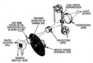
FIG. 4—Simplified view of a mechanical transmitting system.
