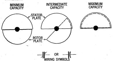
FIG. 11—Arrangement of straight line capacity condensers for various capacities.
