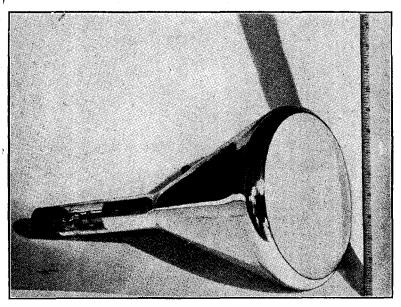
FIG. 10-The kinescope.
