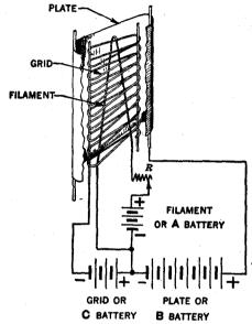
Fig. 14.—Schematic diagram showing triode connection to battery.
