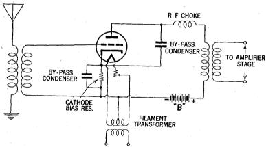
FIG. 25-Grid-biased detector circuit.
