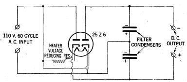
FIG. 17-Voltage doubler circuit utilizing a full-wave rectifier tube.
