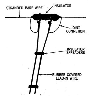
FIG. 20-Illustrating good spacing arrangement for doublet type antenna.
