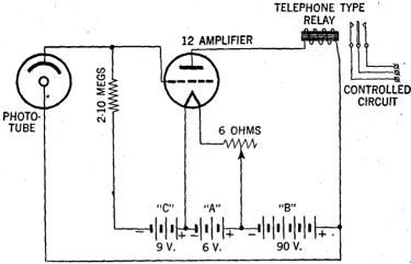
Fig. 42.—Simple battery operated amplifier.
