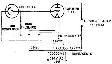
Fig. 6.—Typical A. C. operated amplifier. Reverse circuit for phototube operation.
