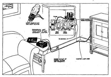
FIG. 13—Diagram of connection when oscillator-phonograph units are employed in connection with receiver for music reproduction.
