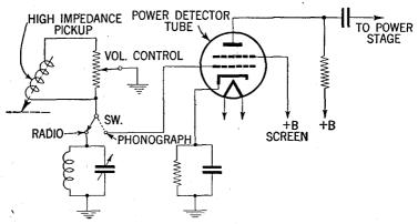
FIG. 9—Conventional method for connection of radio high impedance pick-up.
