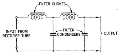
FIG. 6-Choke-input filter.
