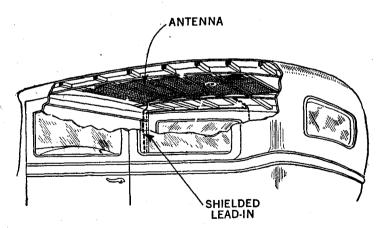
FIG. 2—Illustrating location of roof type antenna.
