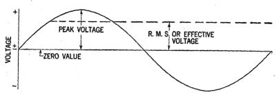
FIG. 44—Illustrating comparative values of r.m.s. and peak voltage in an alternating current.
