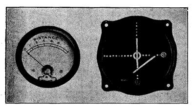
FIGS. 11 and 12—Indicating instrument on the aircraft for utilizing the radio system of landing aids.
