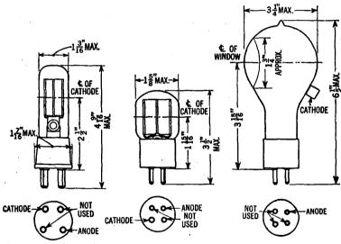
Fig. 6.—External dimension of phototubes shown in fig. 5.
