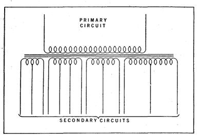
FIG. 2-Typical schematic diagram of power transformer used in radio work.
