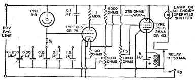
Fig. 20.-A light-quantity metering and control circuit.
