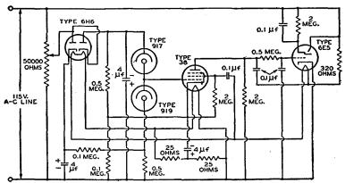
Fig. 21.—A sensitive light-balance indicator.
