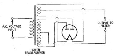
FIG. 5—Illustrates connection and rectifier tube to obtain full-wave rectification.
