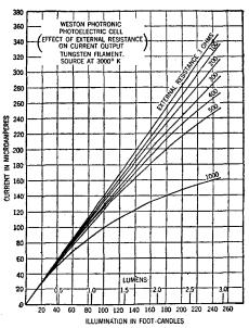
Fig. 15.—Effect of external resistance on current output.
