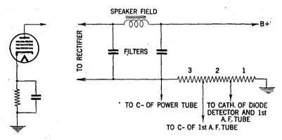
FIG. 39—Showing how grid bias may be obtained by the use of self biased bypassed resistor.
