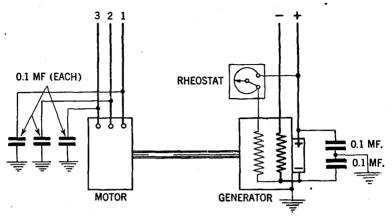
FIG. 5—Interference suppressor arrangement and connection for motor-generator set.
