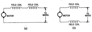
FIG. 2—Diagram indicating how internal connections of a motor may be altered to cause less radiation interference.
