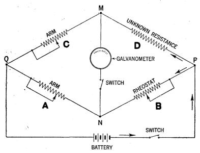
FIG. 25—Schematic diagram of Wheatstone bridge showing resistances and method of connecting galvanometer, battery and unknown resistance.
