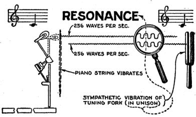
Fig. 3.—Sympathetic vibration of tuning fork with struck piano string when tuned to same putch, illustrating the wave theory of radio.
