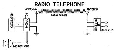
FIG. 1—Diagrammatic representation illustrating similarity between wire and radio telephone.
