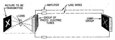
FIG. 3—Diagram of an early television system. At the transmitting end light is converted into electrical energy which when amplified will energize a magnetic shutter or similar device at the receiving end causing a reproduction of the picture. Each photo-electric cell must be individually converted to its correspondingly remotely located light element. In the case under consideration therefore, approximately 80 wires will be necessary.
