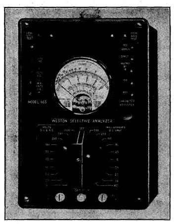
FIG. 13—Typical volt-milliamp-ohmmeter. (Courtesy Weston Electrical Instrument Corp.)
