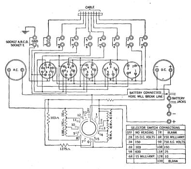
FIG. 33-Connection diagram of Readrite Model 720-A point to point tester.
