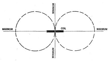
FIG. 1—Illustrating directional effect of radio waves on the loop-antenna part of the radio compass.
