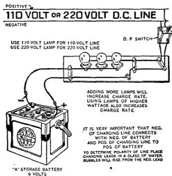
Fig. 20.—Diagram showing method of charging A battery through a lamp bank on 110 cr 220 volt d.c. line.
