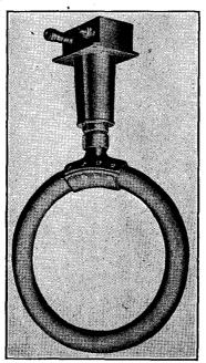
FIG. 8-Aircraft loop-antenna. (Courtesy Western Electric Co. Inc.)
