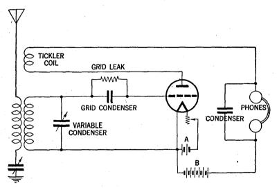
FIG. 17—Regenerative circuit. The scheme of combining a detector circuit with a separate oscillator circuit is called *heterodyning* and oscillators built exclusively for this purpose are called *heterodynes*. A circuit such as this is known as a regenerative circuit, and this term is applied to any detector circuit in which a coupling is provided between the plate and the oscillatory grid circuit.
