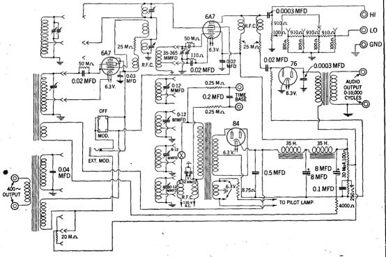
FIG. 29-Circuit diagram of Supreme Model 581 Signal generator.
