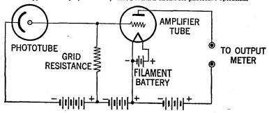
Fig. 4.—Typical battery operated amplifier. Reverse circuit for phototube operation.
