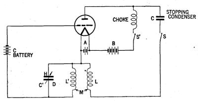
FIG. 6-Modified Hartely type oscillator circuit.
