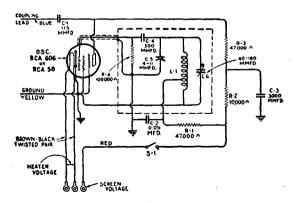
FIG. 14-Schematic circuit diagram of typical oscillator unit.
