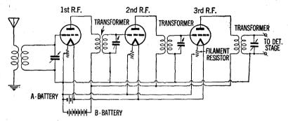
FIG. 14-Three stage radio frequency amplifier circuit.
