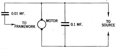
FIG. 1—Schematic diagram showing connection of interference suppressors to a vacuum cleaner.
