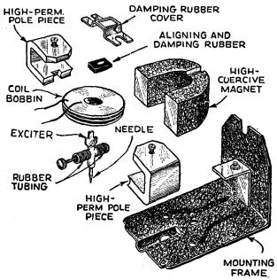
FIG. 4-Parts of modern rubber damped pick-up.
