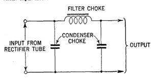
FIG. 7-Condenser-input filter.
