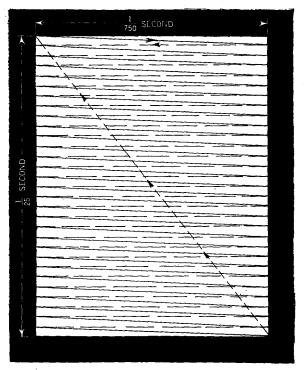
FIG. 17-Simple linear scanning.
