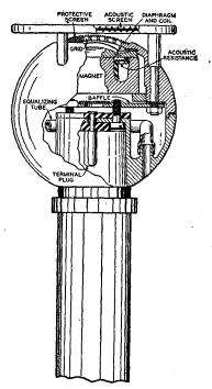
FIG. 20—Simplified cross-sectional view of a non-directional moving coil microphone.
