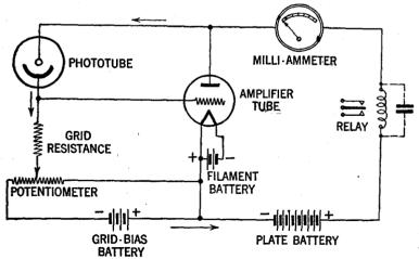
Fig. 2.—Simple battery operated one stage amplifier circuit for use with a photo-electric cell.
