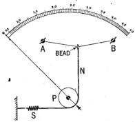
FIG. 16—Simplified diagram illustrating the construction of a hot wire instrument. N, represents a silk thread connected to spring S, wound around pully P, and attached to a bead threaded on wire AB. Wire AB, made of platinum alloy, is connected in the circuit whose current is to be measured. This wire lengthens, due to the heating effect  $(I^2R)$  when a current flows through it. The slack is taken up by spring S, causing pulley to turn and move the pointer over the scale.
