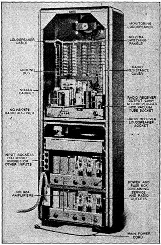
VIG. 8—Rear view of control equipment cabinet shown in fig. 7. Note: The electric phonograph unit is retractable and may be moved back and forth in drawer fashion to facilitate loading and unloading of records. (Courtesy Western Electric Co.)
