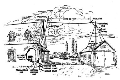
FIG. 2—Typical single-wire antenna installation. (Courtesy R.C.A. Mfg. Co.)
