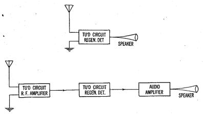
FIGS. 1 and 2—Block diagrams showing essential units of a regenerative and a tuned radio frequency regenerative circuit respectively.
