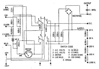
FIG. 36-Wiring diagram of Philco Model 025 radio tester.
