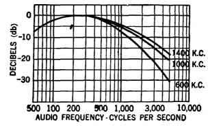
FIG. 8-Typical radio receiver, fidelity characteristics.
