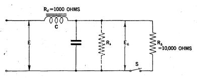
FIG. 16-Showing application of bleeder resistor across power supply.
