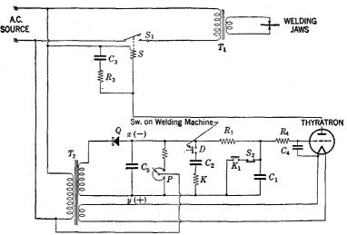
Fig. 5.—Chematic diagram of a low speed welding circuit, with thyratron timer.
