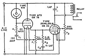
Fig. 13.—A quick-acting A. C. operated photo amplifier relay, functioning in a positive direction on the received light.
