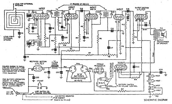
Fig. 28.—Schematic circuit diagram of an A.C.-D.C. portable super-heterodyne receiver. (Emerson DJ-310-311-312.) The circuit has a frequency range of from \$\delta \delta 0\$ to \$1,600 k.c.; contains 6 tubes and can be operated from self-contained batteries as well as from a 110 volt 60 cycle A.C. source. The power consumption is 30 watts. It has a built-in antenna, with provision for connection to an external antenna and ground if desired.
