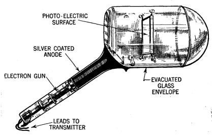
FIG. 11—Another type of cathode ray transmitting tube.
