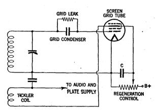
FIGS. 18 and 19—Showing two methods for control of regeneration in radio receivers.
