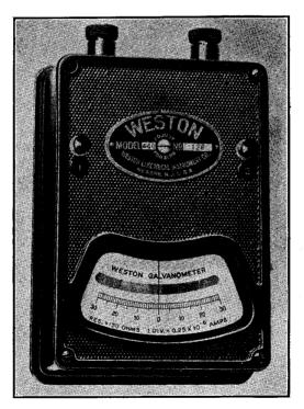
FIG. 4a-Weston model 440 movable coil galvanometer.
