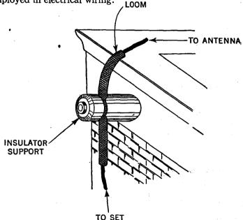
FIG. 6—Demonstrating how a short section of loom is inserted to protect the aerial at the point where the line is supported by a nall-on knob. The loom eliminates swinging and forcing of too sharp a bend in the wire.
