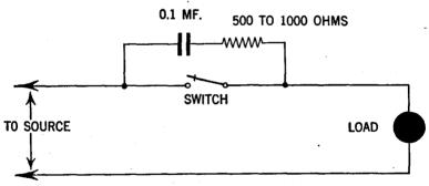
FIG. 6-Method of filter connections across switch.
