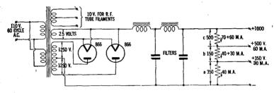
FIG. 11—Full wave rectifier circuit with conventional filters and voltage divider.
