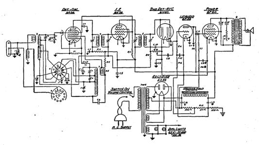
Fig. 5.—Schematic circuit diagram of a 6-tube superheterodyne, 3-band radio receiver. (Zenith Models, 6-S-203, 6-S-223, 6S-229, 6S-239, 6S-241.) I.f. frequency, 456 kilocycles. In locations subject to code interference adjust wave trap marked (E) for minimum interference with antenna connected and receiver operating in broadcast band. Line voltage 117 volts, a.c. 50 to 60 cycles. Power consumption 65 watts.
