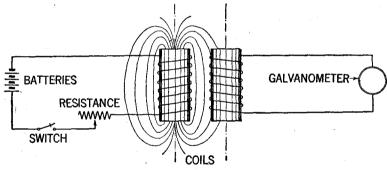
FIG. 7—Diagram showing the action of mutual induction between two coils; the one including a source of electrical energy and a switch, the other a current measuring instrument but having no source of electrical energy. During the increase or decrease in strength of current as on closing the switch the current is induced in the secondary circuit. This secondary current is flowing in a direction opposite to that of the primary current.
