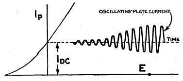
FIG. 7—Oscillating plate current characteristics.
