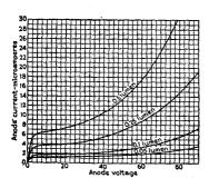
Anode Voltage vs Anode Current for Phototube PJ-23
