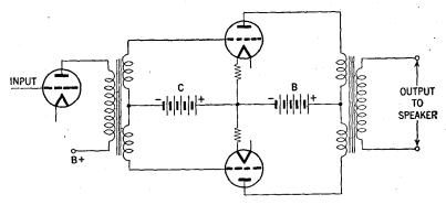
FIG. 15—Push-pull amplifier circuit. This type of amplification requires two identical tubes in each stage. The grids of the tubes are not connected together, as in the case of parallel operation, but are connected to opposite ends of a mid-tapped transformer secondary. The mid tap is used as a common connection for making connection to the negative bias voltage of the grids.
