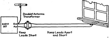
FIG. 7—Showing method of carrying antenna leads through the windows—using either porcelain tubes or flexible lead-in strips. Upper figure shows connections where antenna transformer is embodied in the radio receiver, and the lower, where it is connected outside. Transmission lines must be well insulated and stand off from the walls, as well as kept away from wires, drain pipes and other metallic surfaces and conductors.
