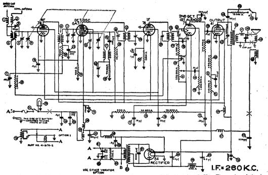
Fig. 6.—Schematic wiring diagram of a 6-tube automobile radio receiver. (Phileo-Nash N-1434-H.) The speaker of the electrodynamic type is designed for mounting on a frame in the center above the windshield. For installation of the receiver mounting holes are provided in the left hand side of the dash. Since all late cars have an all-metal roof it is necessary to install either a cowl extension antenna or an under the car antenna. The under car antenna is installed beneath the running boards.
