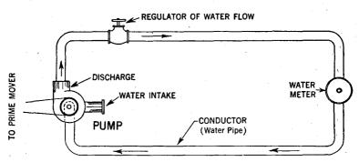
Fig. 6.—Water is forced through the conductor by means of the pump action causing a pressure difference between the conductor terminals.
