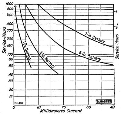
Fig. 2.—Diagram of service hours at various currents from tests made on Burgess dry batteries. Discharge based on intermittent service of 2 hours per day to an end voltage of 17 volts for a 221/4 volt battery.
