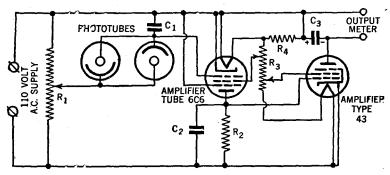
Fig. 25.—Circuit for measurement of light intensity ratios.
