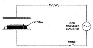
FIG. 14—Illustrating the action of crystal when an electro-motive force is applied.
