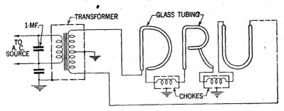
FIG. 9—Typical connection diagram showing interference suppressor arrangement as applied to Neon signs. Chokes, if used, should be of sufficient size to carry the required current without undue heating.
