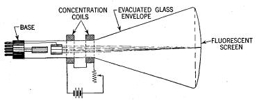
FIG. 12—Cathode ray tube with external concentration coils. The concentration coils generally consists of one or more solenoid of wire placed as shown for focusing the ray. For a practical utilization of this form of ray concentration, however, it is necessary that the position of the coils be definitely fixed and the current through them suitably controlled.
