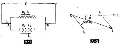
Fig. 16.—Resistance and inductive reactance in parallel combination.
