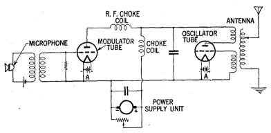
FIG. 5—Circuit diagram showing essential elements for accomplishing plate modulation. In practical installations two or more stages of power amplification is usually interconnected between the microphone circuit and the modulation tube.
