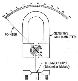
FIG. 17—Schematic thermocouple arrangement and connection to sensitive milliammeter. Note: Unequal division of instrument scale.
