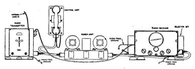
FIG. 3—Marine Radio Telephone equipment. (Courtesy Western Electric Co.)
