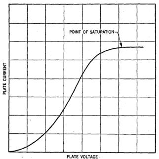
Fig. 13.—Characteristic curve of a diode.
