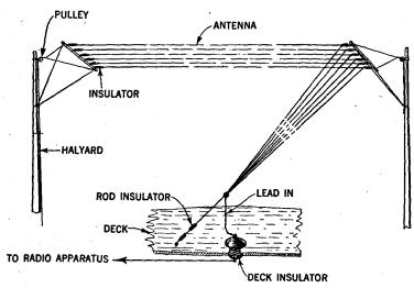
FIG. 6—Ship antenna of the flat-top inverted "L" type, showing conventional method of lead-in and deck-insulator details.
