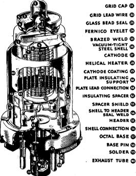
Fig. 3.—Inside view of a metal radio tube. The inside parts are similar to those of a glass radio tube. The housing of the parts consists of metal, which has certain advantages to that of the glass in required electrical shielding. These types of tubes generally are smaller and have a central guide pin projecting from the base for easy insertion in the sockets, and are therefore not as a rule interchangeable with glass tubes. (Courtesy R.C.A. Mfg. Co.)
