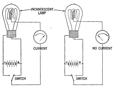
Fig. 5.—Shows how a current will be registered by the galvanometer when the switch is connected to make the insulated plate positive. The current flow, however, will cease when the plate is made negative—the switch connects the insulated plate with the negative terminal of the filament.
