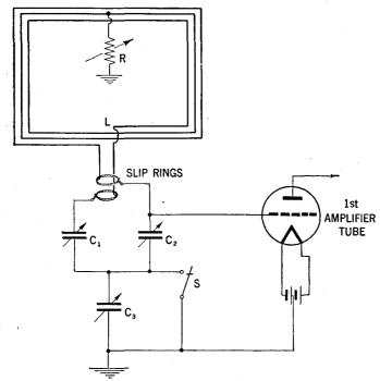
FIG. 5-Circuit of Bellini Radio direction finder.
