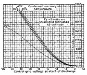
Curves of Anode Voltage vs Controlgrid Voltage at Start of Discherge for Various Condensed Mercury Temperatures for Thyratron Tube FG-172
