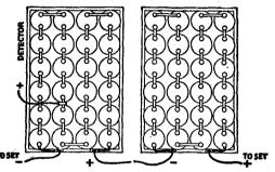
Fig. 27.—Diagram showing two 48 volt B batteries connected in series making 96 volts.
